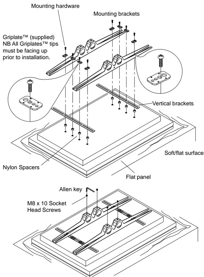
Invert the flat panel display and lay it on a soft and flat surface. Apply the vertical brackets and centre the mounting brackets from left to right on the display. Secure the mounting brackets with the hardware and griplates™ (supplied). NB the griplates™ come with M4, M5, M6 and M8 access holes. Find out what your proper hardware for your flat panel will be and use accordingly.
