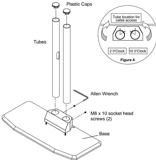
Insert the tubes into the secured aluminium block. See diagram to set the cable access openings before tightening the set screws. See figure A. Once the poles are fully inserted into the block and det to their proper positions lock the tubes by tightening the two.
